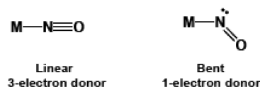
Figure 1. Comparison of a linear three-electron donor \text{NO} group with a bent one-electron donor \text{NO} group.
